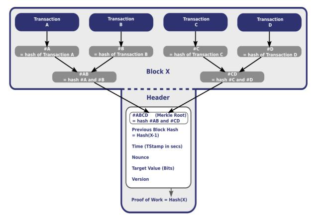
In the blockchain, Merke trees enable to verify a transaction in a much faster way than if a validating a transaction meant recomputing the hash from the whole block data.
