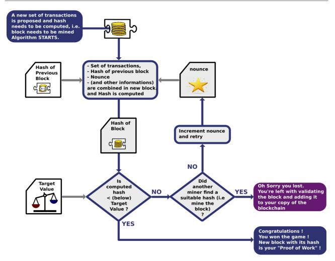
Note 2016.11.21: I should enhance the above schema to illustrate the fact that when a round trip fails, the hash could not be computed, after incrementing the nounce but before retrying, miners add to the current block they are working on the new transactions that they might have received in the meantime. Thus every round occurs potentially on a slightly different block. This is important because it gives its rationality to using Merkle Trees to compute the hash.
